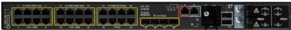
Figure 7. IE-9320-16P8U4X Switch with multi-gigabit and 4PPoE
