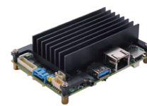
▲ Assembly view for 70°C thermal solution
