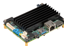
▲ Assembly view for 60°C thermal solution
